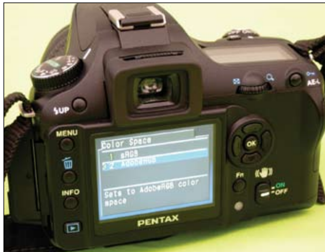
Figure 4: Many digital cameras, including the Pentax K1000 digital SLR shown, have the ability to export files into either sRGB or Adobe RGB working space. For large-format printing, choose the larger Adobe RGB space.
