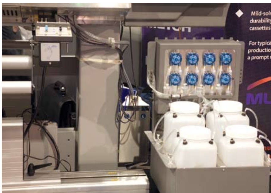
Fig. 3: An optional kit, photographed here, allows a bulk-ink system that will handle 4.3-liter bottles.
