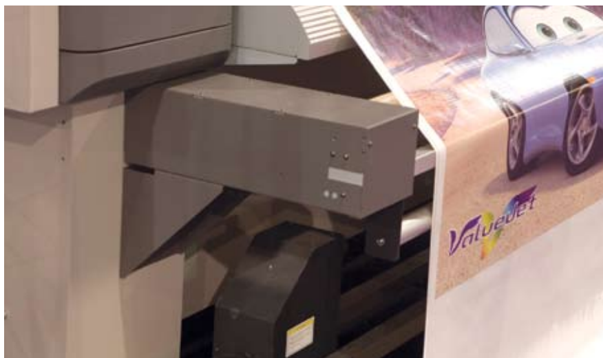
Fig. 5: The 2606's heavy-duty, take-up system can handle up to 220-lb. media rolls.
