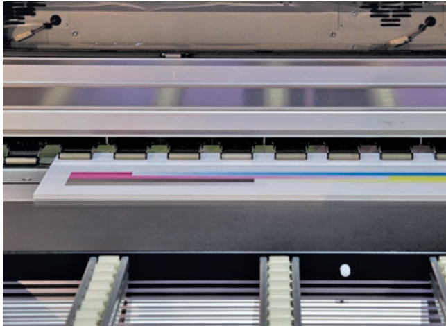
Fig. 1: The system prints and dries the color swatches prior to the color-measurement actions. Note, also, that the printed, measurement pattern spans the media width; thus, it uses minimal media.
